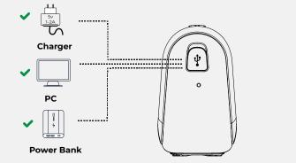
2. When charging, the LED indicator will blink red. When fully charged, the LED indicator will turn off.
