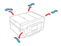
**2** Lift up the scanner unit and remove all protective materials from inside the product.
