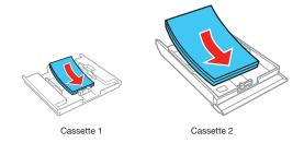
**Note:** Make sure the paper is loaded against the back of the cassette and not sticking out from the front of the cassette.
