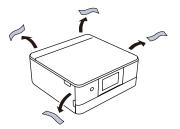
**2** Lift up the scanner unit. Remove all tape and packing materials from inside the product.
