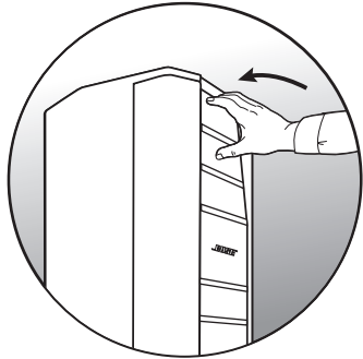
Pushing the array in
