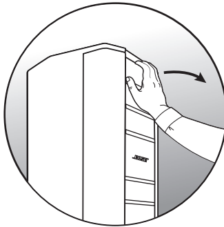
Pulling the array out
