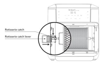
**03** Align the left side of the accessory with the hole in the rotisserie catch, and set the right end of the accessory in the notch on the right. Align the left
