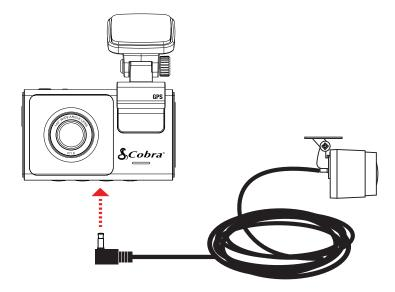
Connecting the FV-CV1 Cabin View Cam
