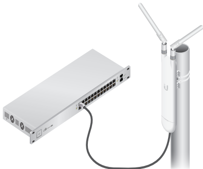
Connected to UniFi Switch, model US-24-250W
