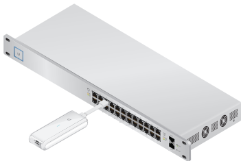
UniFi Switch Power Connection Diagram
