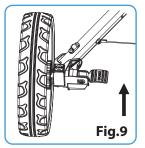
Push on the brake pedal to stop the rear wheel and pull off to release as in Fig.8 and 9.
