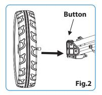
Press the button and insert the rear wheels as in Fig.2
