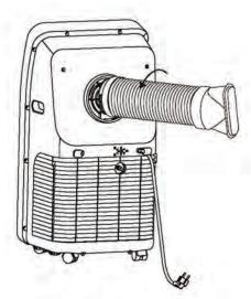
• Insert the air exhaust hose into the window sealing plate, adjust opening width of window so that the window can match with the sealing plate properly; length of the sealing plate is adjustable.
