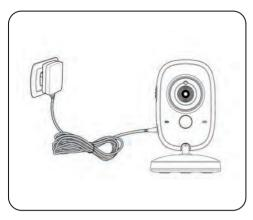
Connect the camera power to the transformer supplied. The blue LED turns on to indicate that it is running.
