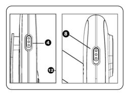
Push the power key up to turn the monitor and camera on
