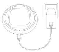
2. Stack batteries on charging base, lining up pogo pins to trigger flashing LED
