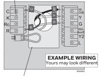
Remove jumper loop ONLY if you have both R and Rc wires.
