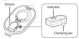
**2** During the re-installation, make sure that the clamping jaw is completely inserted into the groove.
