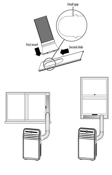
• For optimum performance, do not twist the venting hose. For better efficiency, shorten the hose, if possible.
