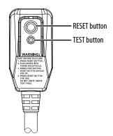
The circuit breaker should be tested periodically by pressing the **TEST** button, then pressing the **RESET** button. If the **TEST** button does not cause the circuit breaker to trip, or if the **RESET** button does not stay engaged, unplug the air conditioner immediately and contact an Insignia technician.
