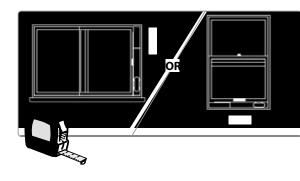
**3** Adjust the length of the window sealing plate to fit the window opening.
