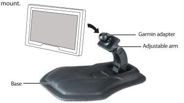
**3** If needed, adjust the viewing angle by tilting your GPS up, down, right, or left. You can adjust the arm up to 90°.
