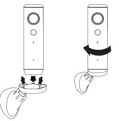
**5** Slide the wall mount onto the wall plate.
