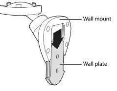
**2** Using the wall plate as a guide, mark and then drill two holes with a 4.2 mm drill bit where you want to mount your camera.
