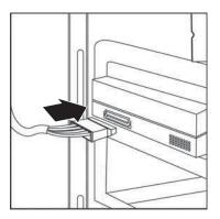
iv The 8-pin PCI-E or 6-pin PCI-E connector to a PCI-E graphic card.
