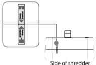
**2** Connect the power cord to a power outlet.
