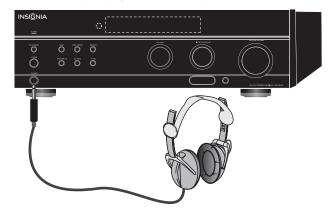
2 Press the SPEAKER A or SPEAKER B button on the remote or the receiver to turn the speakers off. The corresponding speaker indicator turns off, H appears on the display, and sound can be heard from the headphones.
