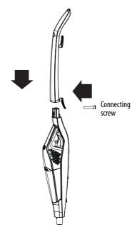
3 Insert the handle/main body assembly into the suction head until it clicks into place.
