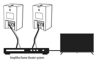
Note: We recommend using 18-gauge or heavier speaker wire.
