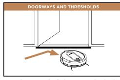
Your robot can easily climb over most thresholds, but if one is higher than 7/8ths of an inch, block it off with a BotBoundary\* strip.
