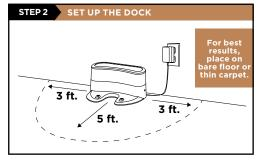
Find a **permanent** location for the dock in a central area with a strong Wi-Fi signal. Remove any objects that are closer than 3 ft. from either side of the dock, or closer than 5 ft. from the front. Place the dock with its back against the wall, and connect the charging cord to the back. The Indicator Light will illuminate green when the dock has power.
