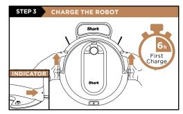
Place robot on dock to charge for 6 hours. Power button must be in the (I) ON position and the robot must be aligned correctly, with its **FRONT** side against the dock. When charging begins, the robot will BEEP and the DOCK light will turn BLUE.
