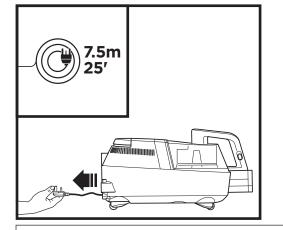
**NOTE:** Hold onto the plug when retracting the cord.
