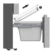
3. Remove the freezer drawer (8) by lifting it up.
