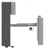
5. Pull out the freezer door and lift it up in the direction of the arrow.
