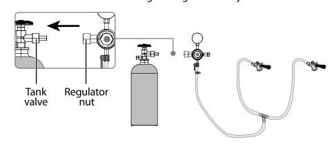
5 Slide the CO<sub>2</sub> tank through the retainer inside the kegerator and secure it with the bolt and nut. Position the tank so that you can read the numbers on the gauge and have easy access to the shut-off valve.
