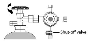
2 Open the shut-off valve to allow gas to flow into the keg.
