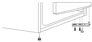
7 Install the leveling foot you removed from the left side into the right bottom of your refrigerator.
