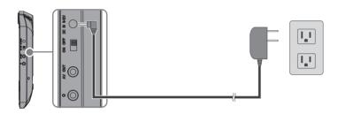
2 The battery charging indicator turns solid green when the battery is fully charged. Unplug the AC power adapter to use your player with the built-in battery.
