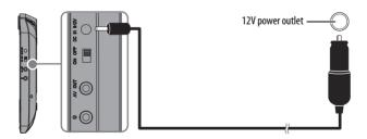
2 The battery charging indicator turns solid green when the battery is fully charged. Unplug the 12 V DC vehicle power adapter to use your player with the built-in battery.
