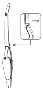
2 Insert the handle/main body assembly into the suction head until it clicks into place.
