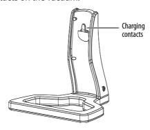
2 Plug the charger into a wall outlet and into the charger stand. The LED blinks (every two seconds) to indicate that the vacuum cleaner is charging.
