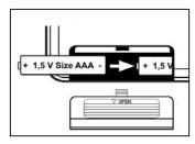
Slide the included 3 AAA batteries into the battery compartment located underneath the scale. Ensure +/- terminals are correctly oriented. When replacing the batteries, please use a small tool to help remove the battery from the battery compartment if necessary.
