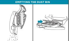
During the first few weeks of use, the dust bin will need to be emptied more frequently, as your robot will now be removing dust and debris from areas that were previously hard to reach. Empty debris and dust into trash.
