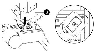
**3** Attach the leg to the desktop with four M6  $\times$  16 screws, tightening them firmly with the 4  $\times$  4 Allen key.
