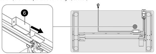
2 Connect the cable from the switch to the adapter cable **6**, then lock them together (see detail).
