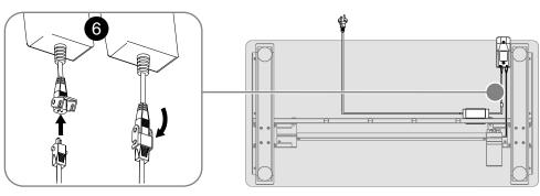
3 Plug the small connecter on the power cord into the female connector on the adapter (see detail).
