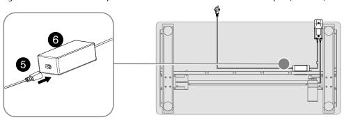
4 Connect the adapter cable 9 to the DC port. Connect the motor cable to the M1 port (see detail).
