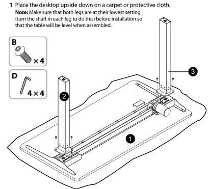
2 Insert the hexagonal shaft in the first leg 3 into the corresponding hole in the desktop leg mount, then turn the leg until the screw holes line up and the connecting cable on the top of the leg faces the in toward the motor.
