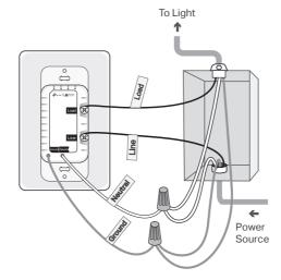
Line up the switch with the mounting holes. Secure it with screws.
