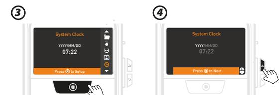
On **SYSTEM CLOCK** screen, press **SHUTTER BUTTON** to set date and time.
