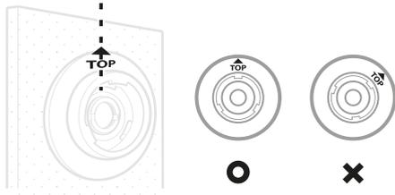
4. Use the tightening tool to tighten the peephole barrel.
