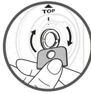
5. Remove the protective film from the lens of the camera.
