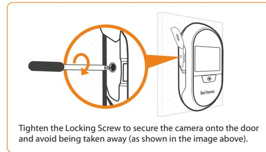
Tighten the Locking Screw to secure the camera onto the door and avoid being taken away (as shown in the image above).
