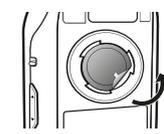
6. Attach the camera to the flange. Rotate it clockwise and lock the camera.
