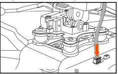
d. Plug both data cables into the corresponding plugs near the Skyview HD Quadcopter's on/off switch
