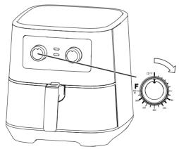
4 Turn the timer knob to set the cook time (from 0-60 minutes) and start heating. The power and heat indicators light and the timer starts counting down from the set cook time.
