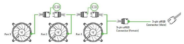
7. Link one of the fans (Fan 1) to the 12-pin breakout cable using the 4-pin PWM connector, and then link the other fans in sequence using the 3-pin PWM connector.
