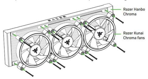
5. Mount your radiator inside the PC chassis then fasten it from the outside using the washers and the radiator screws.
