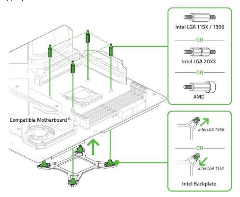
3. Align the AIO cooler with the standoff screws then secure it using the thumbscrew caps.
