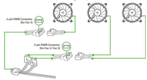
8. Connect the USB Type-C cable and 12-pin breakout cable to your AlO cooler. Attach the rest of the connectors to the CPU fan header and USB 9-pin header of your motherboard; and the SATA cable from your power supply respectively.
