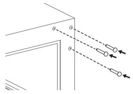
**14** Use a thin, flat blade screwdriver or knife blade to remove the three black decorative plugs from the top left hinge holes.
