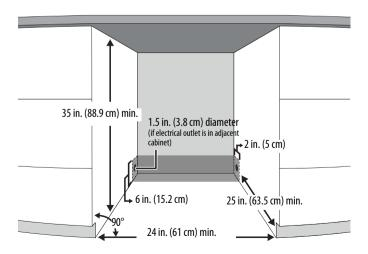
If you are installing your cooler between frameless cabinets, a 0.5 in.(1.3 cm) wide filler strip or side panel may be needed on both sides of your cooler. The filler strip provides a space between the appliance case and the adjacent cabinet door swing. The width of the opening must include the filler panels. The door should extend at least 1 in. (2.6 cm) beyond the surrounding cabinets.
