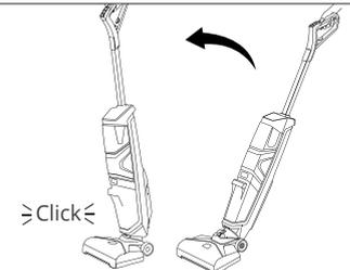
Finish cleaning. Press the power button or push the handle bar forward until you hear a click. The vacuum automatically turns off. Note: After you press the power button, it will take 5 seconds for the vacuum to stop cleaning.
