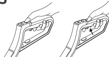
Press the Power button to start cleaning. Press the speed control button to select a rotation speed: High / Low. Press the water spray button. Water and floor cleaner will spray onto the rolling brush.
