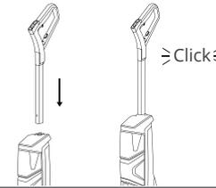
Insert the handle bar into the main body. You will hear a click when the handle bar is locked in place.
