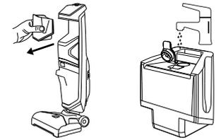
Remove the clean water tank, open the rubber cover, and add water. Note: Use 2 bottle caps of floor cleaner for best results.
