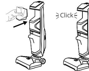
Replace the clean water tank. You will hear a click when the water tank is locked in place.
