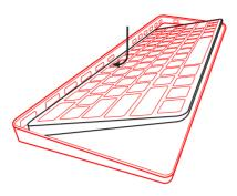
3 Snap front edge of keyboard into MagicBridge to secure in place.
