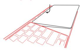
5 Snap front edge of trackpad into MagicBridge to secure in place.
