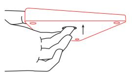
2 Then push up from bottom, and pull front tab forward at the same time slightly to release.
