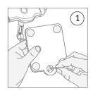
Remove Arm Attachment Bolt from bottom of Base and release HoverBar Arm
