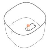
2. Align the rear end of the water pipe with the rotator and press down until it locks in place tightly.
