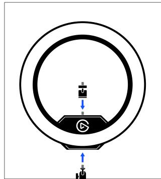
**2.** Secure Ring Light to the 1/4 inch screw on top of the ball head. Extend Master Mount S to your preferred height.
