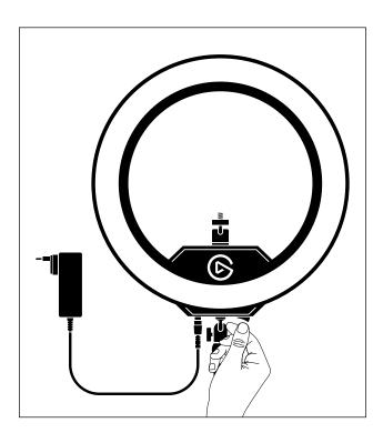
**3.** Connect the power supply and plug it into a power outlet. Switch on Ring Light. It will take approximately 10 seconds to boot up.
