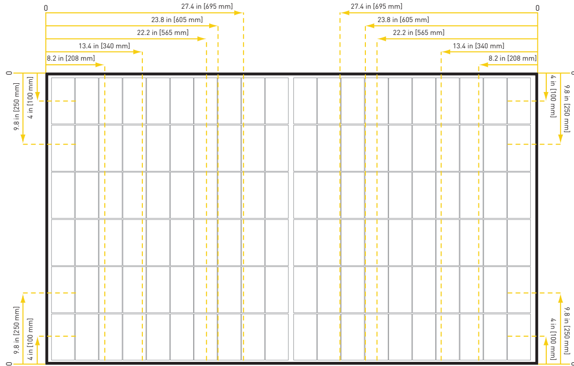
Figure 9. Clamping of EVPVxxx and EVPVxxxK Series modules with rails parallel to short side of the module
