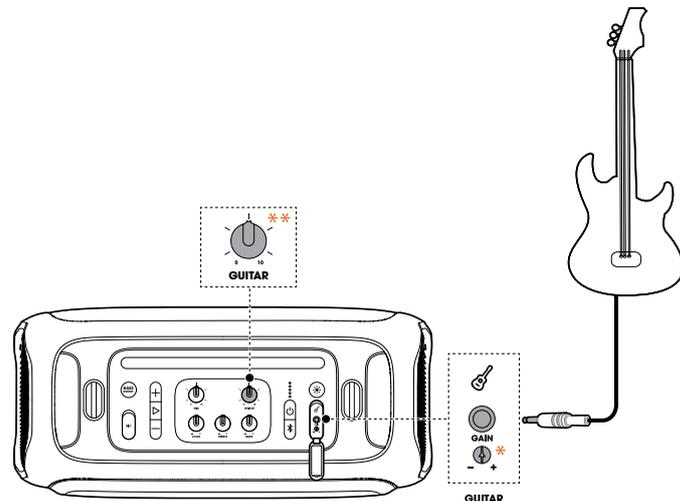
**EN** \* Rotate to adjust the guitar gain.
