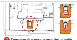
Remove the screw and the plastic piece from print bed.
