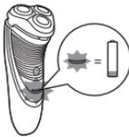
When the battery is almost empty, the charging light starts to flash red.
