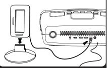
Snap AM antenna into provided stand, then plug antenna cable into socket on back of iP90. Move antenna 12" away. Extend FM antenna.
