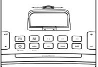
Press the Radio button and press again to select AM/FM band. Press the + or - button to tune in a station. See page 4 for programming presets.
