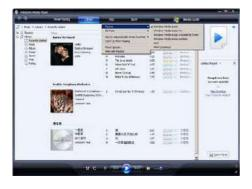
4 Click on the down arrow beneath the **Rip** tab and select the **Bit Rate**.
