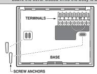
NOTE If you are mounting the base to a soft material like plasterboard or if you are using the old mounting holes, the screws may not hold. Drill a 3/16-in. (4.8mm) hole at each screw location, and insert the plastic anchors provided. Then mount the base as described below.
